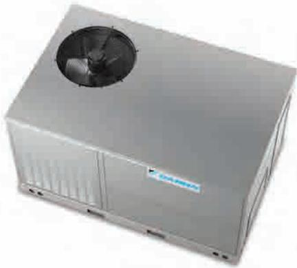
The Daikin DT High-Efficiency Commercial Packaged Air Conditioners and Heat Pumps feature a high-efficiency scroll compressor, high-capacity steel-cased filter drier, and easy access for servicing. These units are housed in a heavy-gauge, galvanized-steel cabinet with UV-resistant powder-paint finish.
