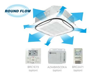
Together with the occupancy sensor, the air-temperature sensor and the built-in surface temperature sensor are used to maintain an even and comfortable temperature distribution from floor to ceiling in the room. This is done by automatically adjusting the supplied airflow rate and the individual position of each of the four supply air louvers in the unit, thus maintaining the required comfortable space environment.
