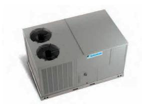
The Daikin DCG Commercial Packaged Gas/Electric Units feature the chlorine-free refrigerant R-410A. Other features include our dual-diameter tubular heat exchanger and a high-efficiency scroll compressor. These units are housed in a heavy-gauge, galvanized-steel cabinet with UV-resistant powder-paint finish.
