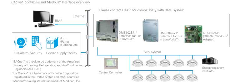
Daikin's *BACnet*, *LonWorks* and *Modbus* interface units provides control for all *VRV* systems.
